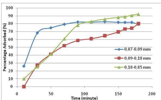
Fig. 1. Effect of contact time and different particle size of LABSA on removal efficiency: 100 mg/L LABSA solution, 0.1 g/100ml adsorbent dose, pH 7, T= 25 °C
