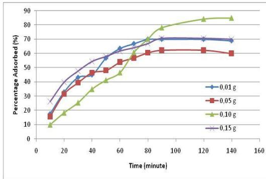
Fig. 5. Effect of contact time and adsorbent amount of LABSA on removal efficiency: 100 mg/L LABSA solution, particle size 0.18-0.85 mm, pH 7, T= 25 °C
