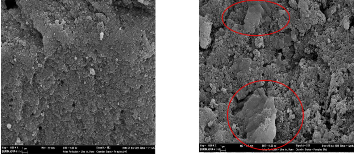
Fig.9 SEM micrographs of char at mag. 10.000 (left: char and right: adsorbed char)
