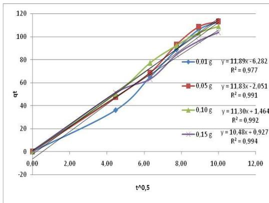
Fig. 7. Intra-particle diffusion plot for adsorption of LABSA on Char : 100 mg/L LABSA solution, 0.01 – 0.05 - 0.1- 0,15g/100 ml adsorbent amount, pH=7, particle size 0.85-0.18 mm, T=25 °C
