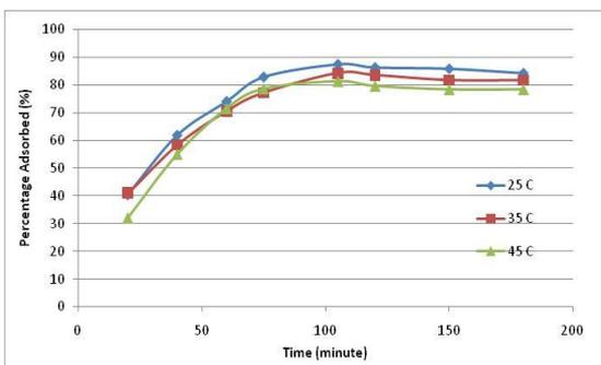
Fig. 3. Effect of contact time and temperature of LABSA on removal efficiency: 100 mg/L LABSA solution, 0.1 g/100ml adsorbent dose, particle size 0.18-0,85 mm, pH=7
