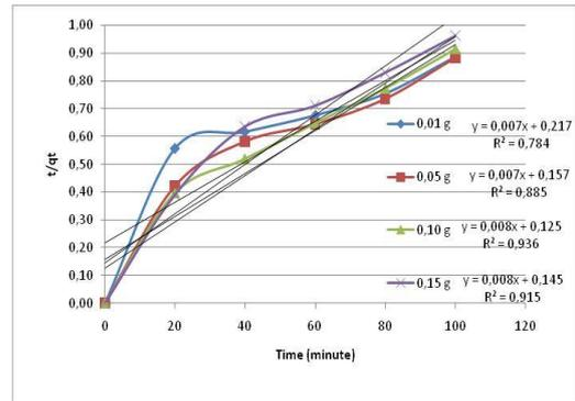
Fig. 6. Pseudo-second-order plot for adsorption of LABSA on Char : 100 mg/L LABSA solution, 0.01 – 0.05 - 0.1- 0,15g/100 ml adsorbent amount, pH=7, particle size 0.85-0.18 mm, T=25 °C
