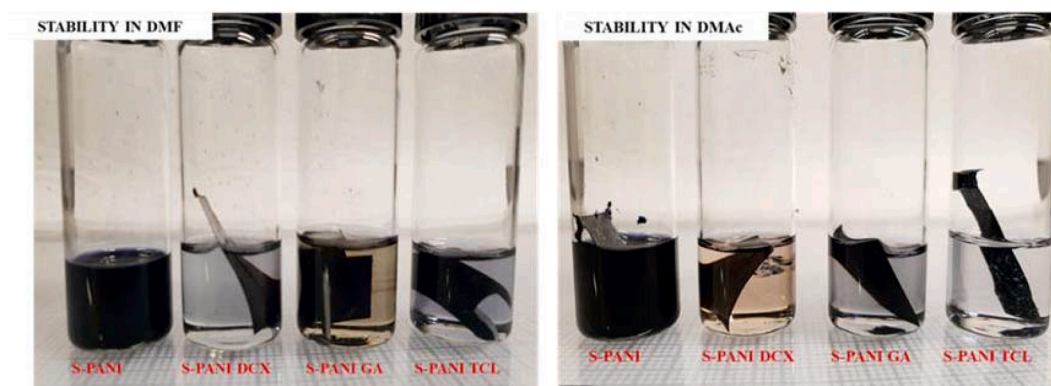
Fig. 8. Effect of DMF and DMAc on membrane stability. Picture is taken after half an hour from immersion in solvents.
