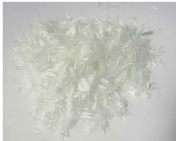
FIG. 1. Representative image of as-received state of the glass fiber waste. [Color figure can be viewed at wileyonlinelibrary.com ]
