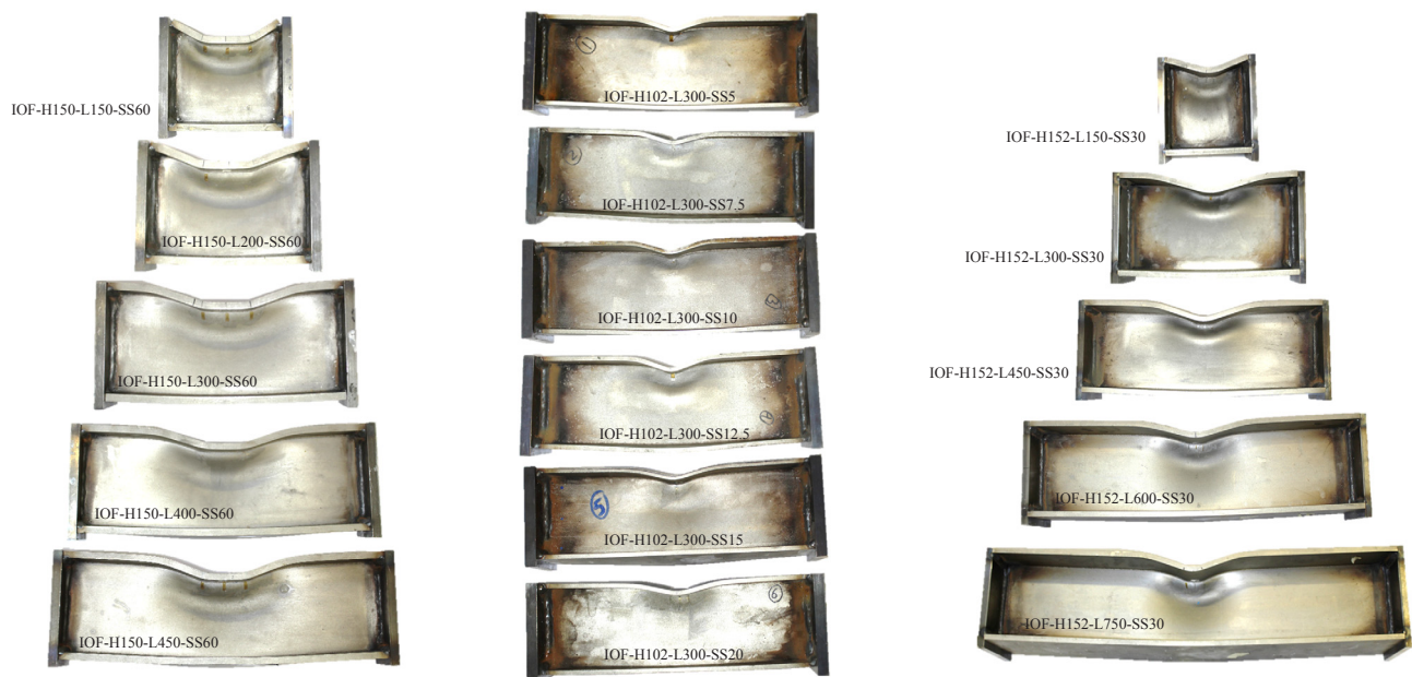
Fig. 5. Failure modes of internal one-flange (IOF) loading test specimens.
