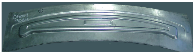
Fig. 5 A DP600 steel roof-stiffener part
