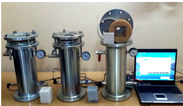
Fig. 2 The setup of the modified permeameter test apparatus
