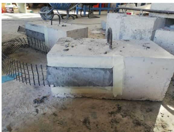
Taping around the strip
