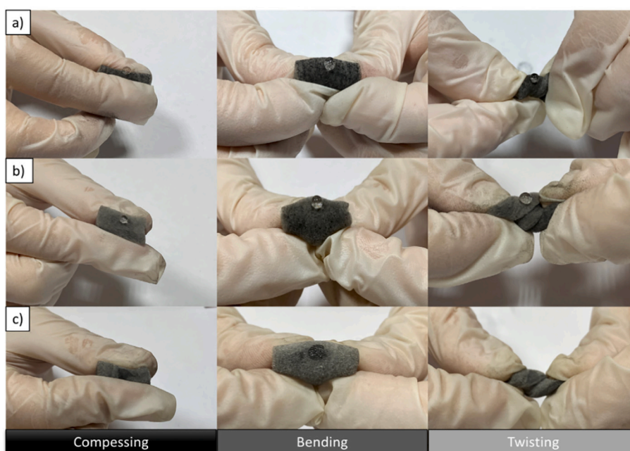
Fig. 11. Mechanical stabilities of (a) coated sponge, (b) after acid, and (c) alkali treatment.
