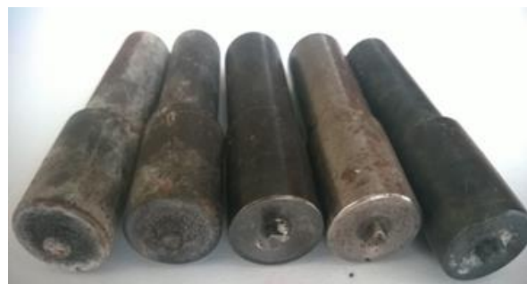
Fig 2.3 48CrMo 6 7 It is made of hot work tool steel friction stir tools.
