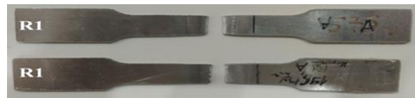
Fig 2.19 Tensile specimen after fracture; the FSW accomplished at tool rotational velocity of 1600 rpm, tool traverse speed of 125 mm/min (ASTM E8M-04).
