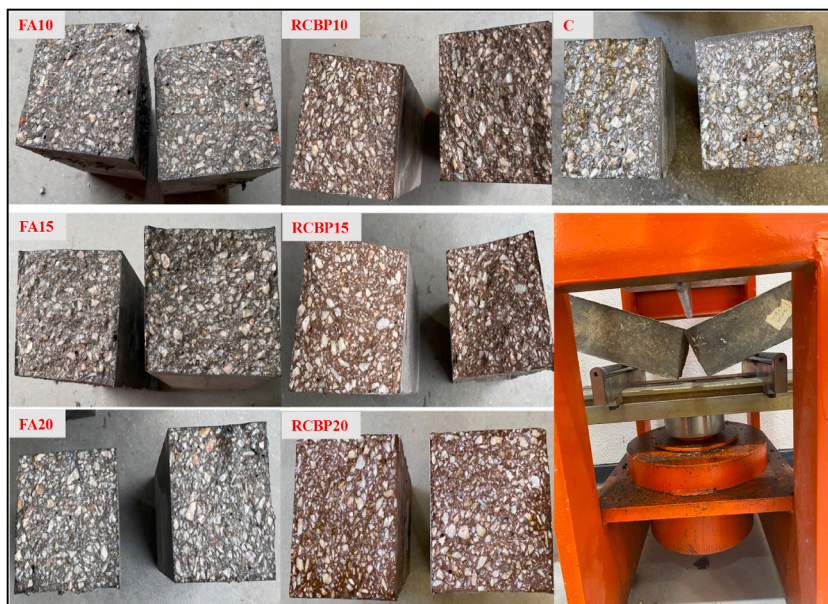
Fig. 14. Cross-sectional views of HSSCC series (90 days) after fracture under flexural strength test.
