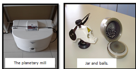
Figure 1. Photographs of the planetary mill, jar and balls.
