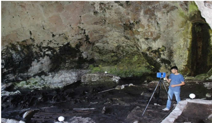
Figure 13. Scanning of wooden floors with a laser scanner.
