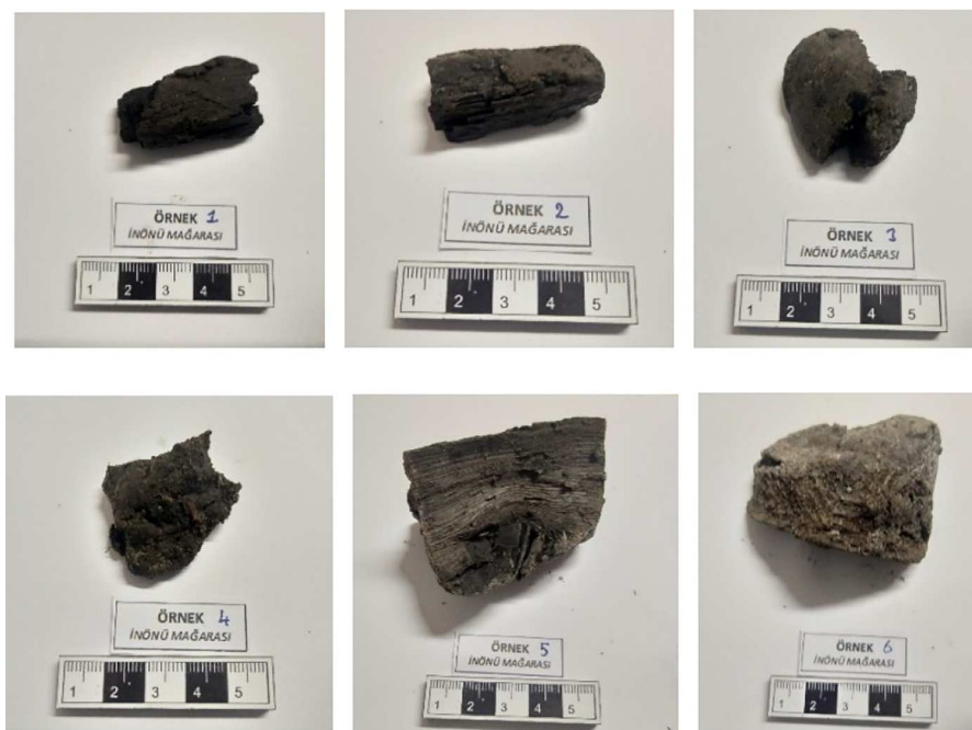
Figure 9. Wood samples whose textural structures were examined by looking at the wet-dry weight difference.
