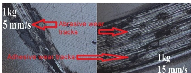
Figure 10. Optical microscope images of the plasma nitrided sample at 450 °C at the 1 kg load, 5 and 15 mm/s sliding velocity by ball-on-disc tribometer.
