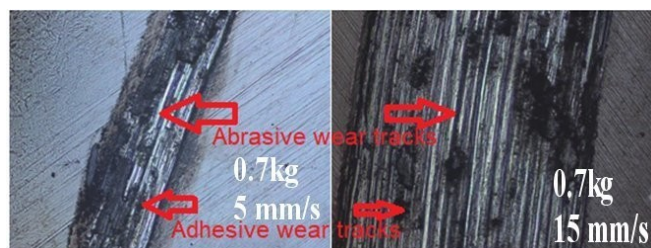
Figure 9. Optical microscope images of the plasma nitrided sample at 450 °C at the 0.7 kg load, 5 and 15 mm/s sliding velocity by ball-on-disc tribometer.
