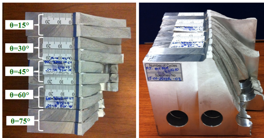
Fig. 18. Broken sample pictures and fracture surfaces of CTS-specimen for different loading angles performed [31,32].
