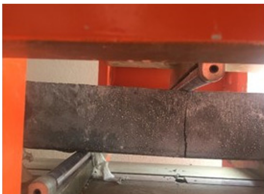
Figure 4: Flexural test on the sample.
