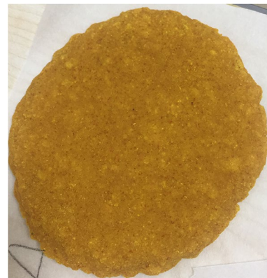
Fig. 4 Green composite sound insulation material (GCSIM)
