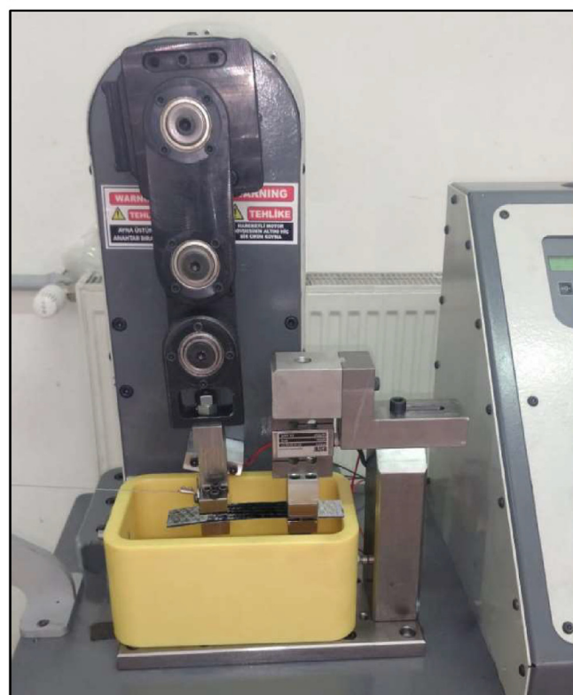
Fig. 4. Working principle of the plane bending fatigue testing machine.
