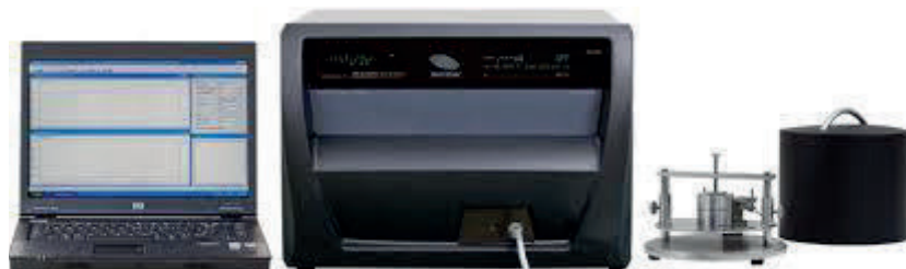
Figure 3 HotDisk TPS2500S Thermal Conductivity Measurement Device( Hot Disk Instruments, n.d. )
