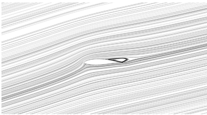
Fig. 10. Flow separation over the blade profile for \alpha = 15^\circ and Re = 7 \times 10^5 .
