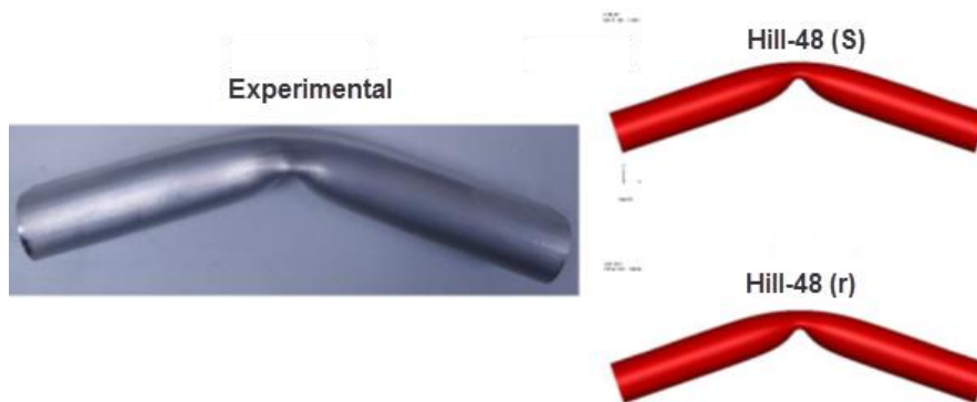
Fig. 10. Comparison of experimental and finite element analyzes of profile with elliptical section geometry with 200 mm span distance and 5 mm punch radius
