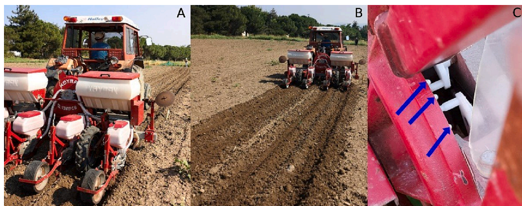
Fig. 3. Sowing EPN capsules with a precision planter (A, B) and capsules on the seed plate (C, blue arrows). (For interpretation of the references to colour in this figure legend, the reader is referred to the web version of this article.)
