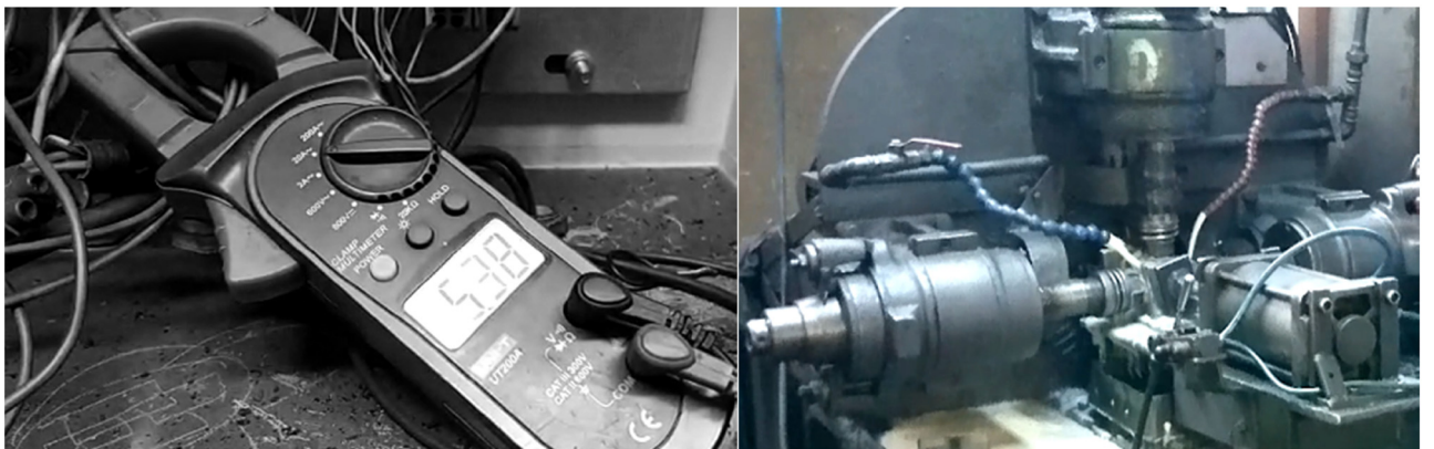
Figure 2: Current index measurement with ammeter (left), Bench where experiments are carried out (right).
