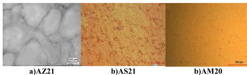
Fig.1. Optical Micrographs of a) AZ21, b) AS21 and c)AM20 magnesium alloys.
