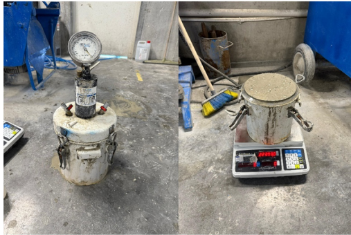
Figure 1. Concretes prepared for determination of fresh concrete unit volume weight
