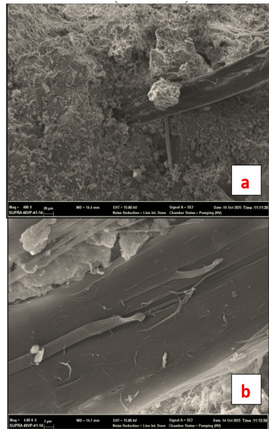
Figure 15. Recycled fiber appearance in sample F10-2 (400 and 4K)
