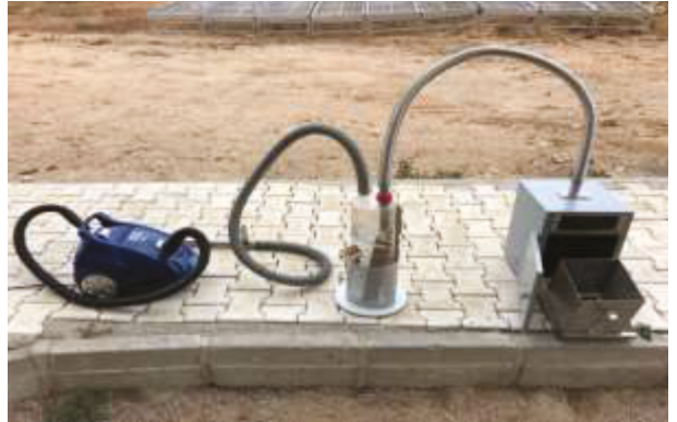
Figure 1. Special system used to obtain the smoke solution.
