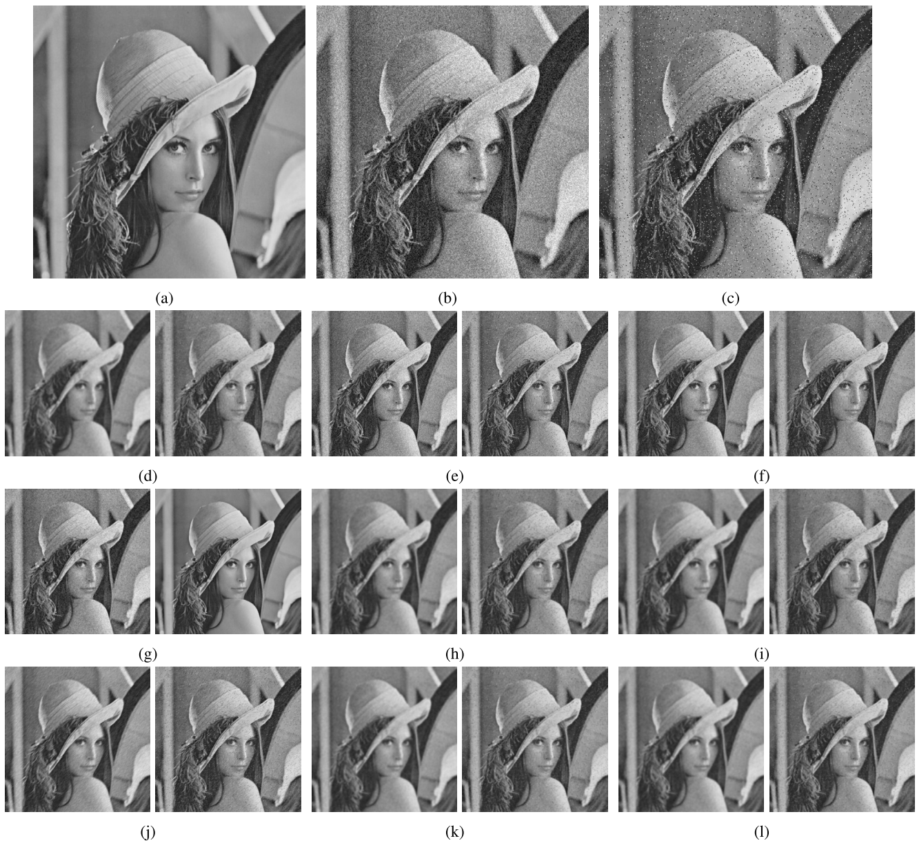
Fig. 2. Gauss noise (left) and Salt-Pepper (right) reduction results: (a) Original, (b) Gaussian noisy image, (c) Salt-Pepper noisy image; Isotropic filters: (d) Beltrami, (e) Gauss, (f) Mean, (g) Median; Anisotropic filters: (h) New Randers, (i) Ingarden, (j) N. Miron, (k) New N. Miron, (l) New Metric.
