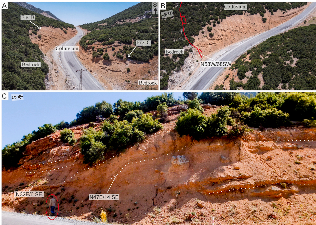
Fig. 16. A. Images showing the road-cut exposures along the valley east of landslide LsSW2. See Figs. 13 and 14 for location. B. Image of the eastern road cut showing angular colluvial deposits (talus) in fault contact with limestone. C. Image of the western exposure showing a monoclinial fold on alluvial fan deposits ascribable to a buried S-dipping secondary fault. Red circle indicates person for scale.
