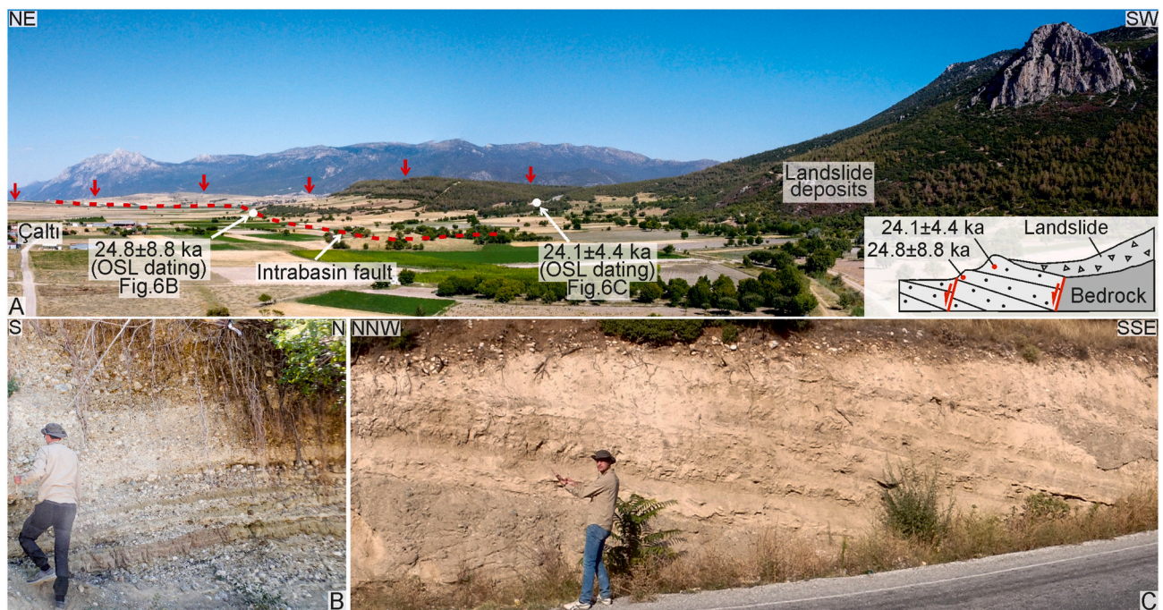
Fig. 6. A. Image showing the intra-basin fault scarp in the southwestern part of the Acıgöl Graben. The red arrows point to the trace of the main fault along the mountain front, locally covered by landslide deposits. A red dashed line delineates the intra-basin fault that offsets the basin deposits. Location of the OSL samples is marked within the image. Inset sketch illustrates the relationship between the faults, the dated basin fill sediments with growth stratal geometries, landslide deposits at the basin margin and the carbonate bedrock. B. Image of the outcrop situated at the base of the intra-basin fault scarp. The southward dip is observed in the gravel deposits with intercalations fine-grained beds. C. Image of the outcrop situated at higher stratigraphic position with S-dipping gravel and sand beds.
