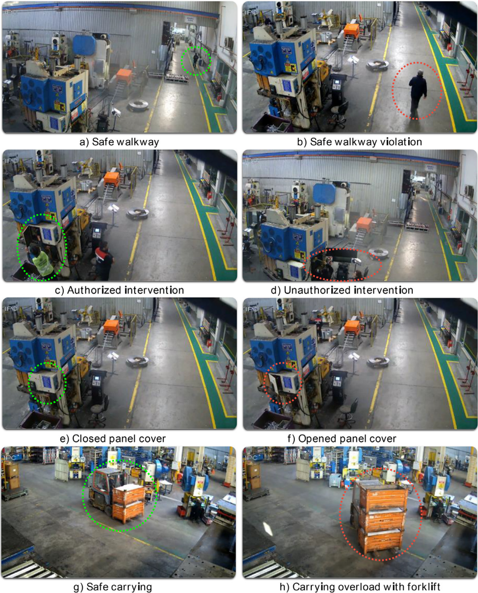
Fig. 1. Example frames of safe and unsafe behaviour video clips in the dataset.
