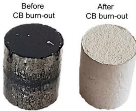
Fig. 3. The representative photographs of the alumina samples before and after removal of CB phase.
