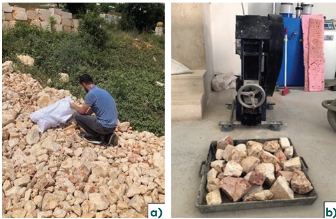
Figure 3. a) marble quarry supply of marble waste; b) material crushing with the help of mini crusher
