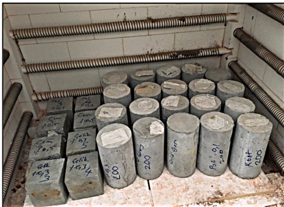
Fig. 4. The heating process in the high-temperature furnace.
